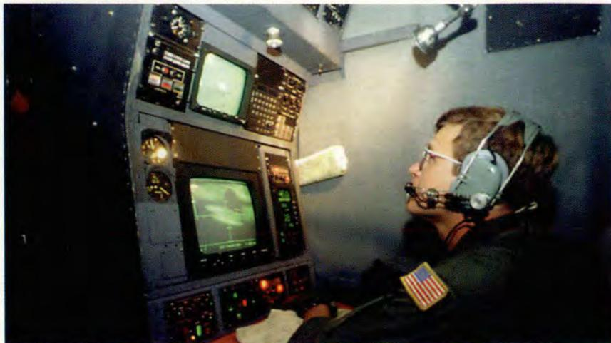
The Air Force has fielded numerous weapon systems with a night capability. NVG (top) and FLIR (above) devices are two of the more common systems used.
